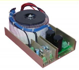
This power supply is designed for used in the Step/Servo motor drive and high over loaded applications. It will work on both standard 115V and 230V at 50Hz or 60Hz. This toroidal transformer has heavier gauge wires then the normal requirement to avoid the copper lost during the full load output and over load output.
