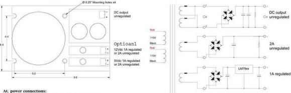
115Vac -2 red wires to neutral & 2 black wires to hot. 220Vac -1<sup>st</sup> red wire to neutral, 1<sup>st</sup> black wire to 2<sup>nd</sup> red wire, and the 2<sup>nd</sup> black wire to hot.
