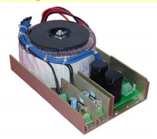
This power suppliy is designed for used in the Step/Servo motor drive and high over loaded applications. It will work on both standard 115V and 230V at 50Hz or 60Hz. This toroidal transformer has heavier gauge wires then the normal requirement to avoid the copper lost during the full load output and over load output.
