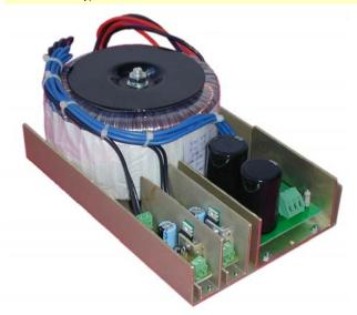
This power supply are designed for used in the Step/Servo motor drive and high over loaded applications. It will work on both standard 115V and 230V at 50Hz or 60Hz. This toroidal transformer has heavier gauge wires then the normal requirement to avoid the copper lost during the full load output and over load output.
